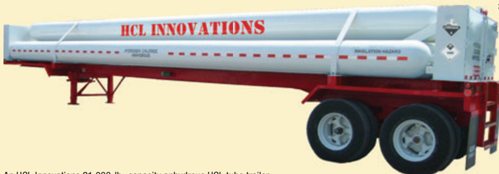
An HCL Innovations 21,000-lb.-capacity anhydrous HCL tube trailer.
